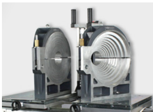
Cast-aluminum clamping jaws
