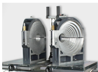
Cast-aluminum clamping jaws
